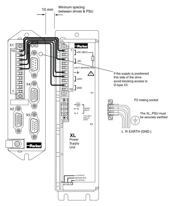
Figure 3-3. XL Power Supply and Drive Connections
